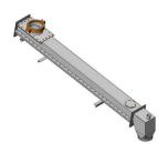
The Air Shoot is an incredibly simple yet effective low pressure, air-activated gravity conveyor for transferring fluidizable materials. Material is moved in a near horizontal plane with minimal changes in elevation for layouts with low headroom or small vertical height differential between source and destination points. Available in open and closed (dust free) models and can be manufactured to your specifications.
